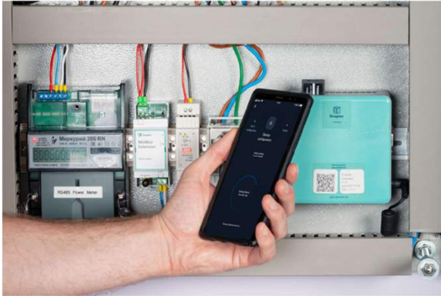
Figure 7: The Enapter gateway being provisioned using the mobile application
